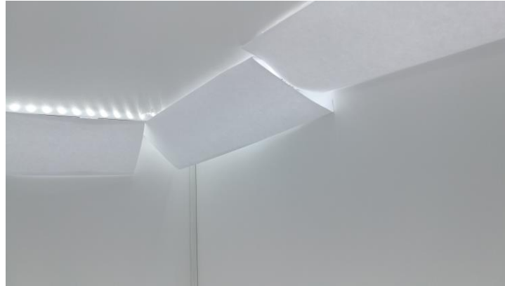
Figure 5.18 Light diffusers simulation with high-density paper sheets
