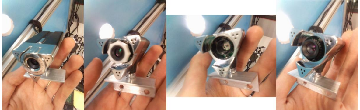
Figure 5.21 Camera lens changing procedure. From left to right: normal webcam, webcam with the focusing wheel detached, webcam with the lens detached (only the camera sensor remaining), webcam with the new lens attached
