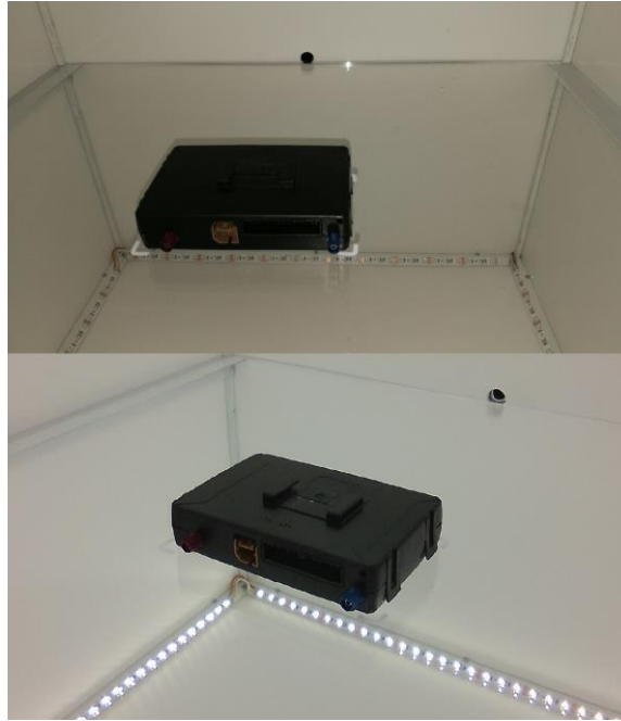
Figure 5.11 MEC prototype's interior, with a transparent support, LED strips and panel holes for the cameras. The upper image shows a TCU with the LEDs off, while the lower image shows a TCU with the LEDs on
