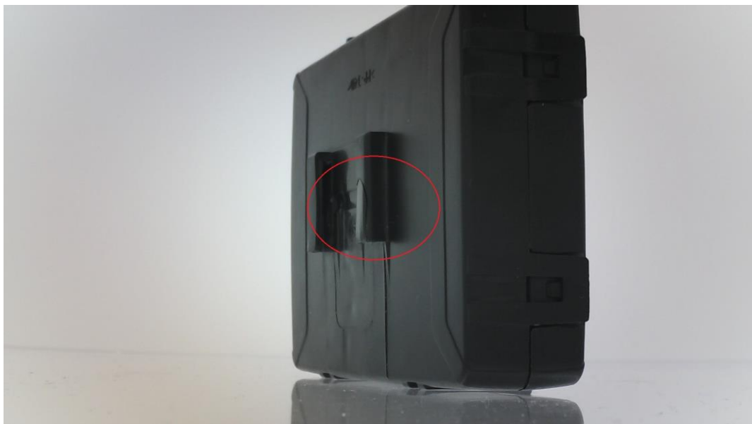
Figure 5.25 Crack in the union between test sample and mechanical test bracket
