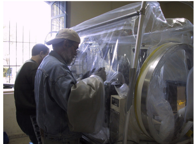
Fig. 3 Generation of samples from drilling cores in strict anaerobic and sterile conditions using a N_2:H_2 gas mixture for an efficient removal of O_2
