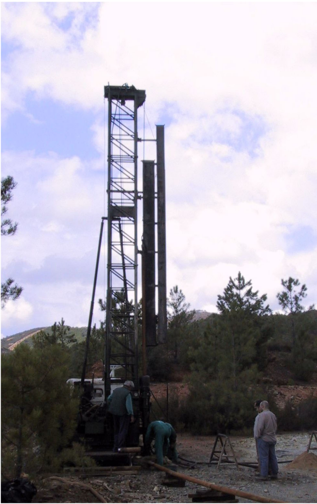
Fig. 1 Sampling the deep subsurface of the Iberian Pyrite Belt using drilling and coring techniques
