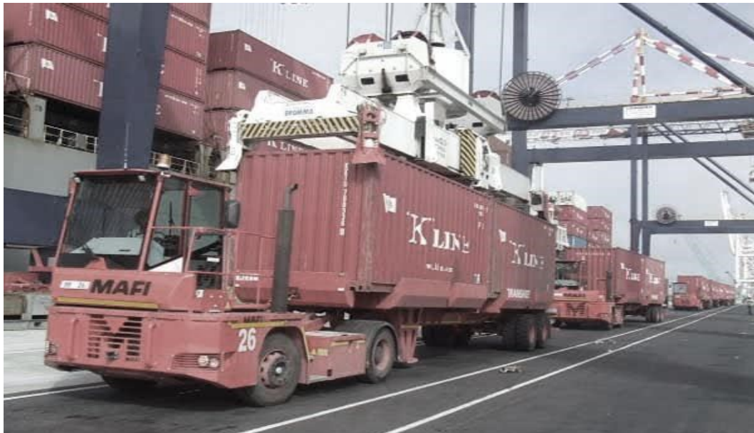
Figure 5-25: Internal hauler and bathtub trailer at the CTCT
