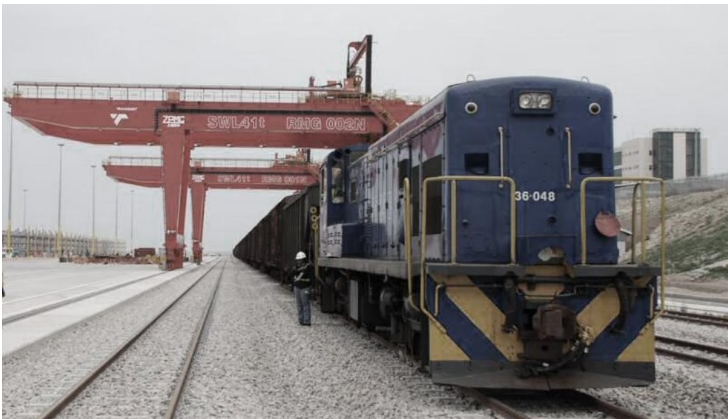
Figure 5-23: Example of rail mounted gantry crane (RMG crane) at Coega Port
