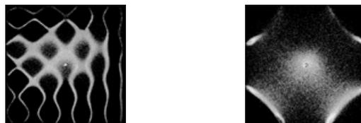
Fig. 2. Cymatic Effect observed through sand on vibrating plate.
