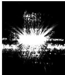
Figure 7: Image of laser reflection on metallic part
