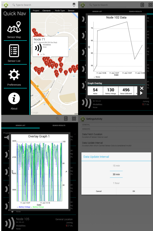
Fig. 2. Selected screenshots of Sensorem . Clockwise from top left: Sensor Map with quick navigation menu; Sensor List with single data graph; Overlaid graph; Preferences screen.
