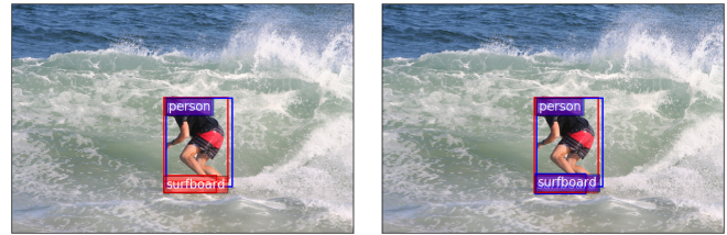
Figure 4: Two scenes from MSCOCO15 (best viewed in color). In each scene, the left image contains the output of the baseline method FRCNN, whereas the right image contains the output of our proposed KG-CNet. Ground-truth objects are marked with orange boxes, and correct detections of IoU at least 0.75 in top 100 are marked with blue boxes.
