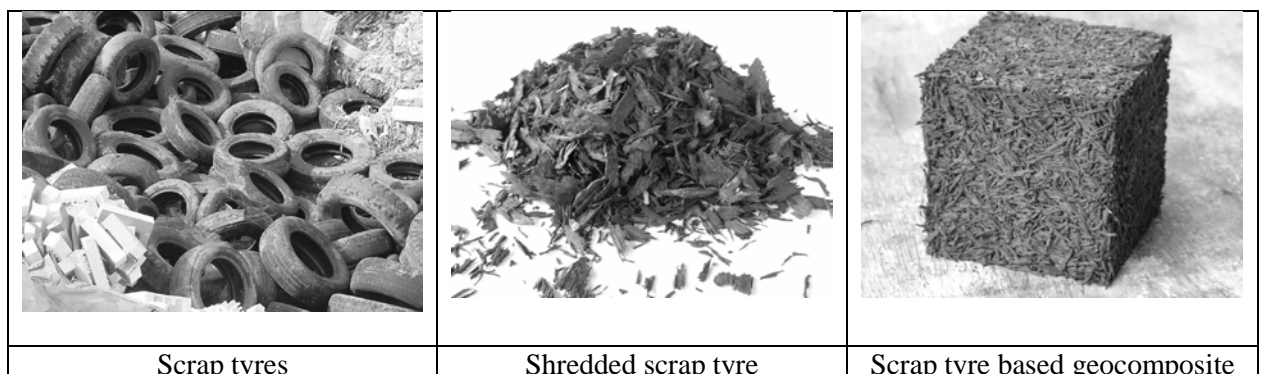
Figure 4: From scrap tyre to block geomaterial
