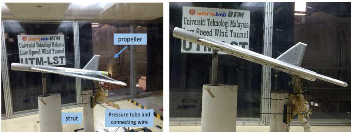
Fig. 6. Installation of UTM-LST sharp-edged delta wing UAV model
