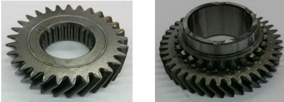
Fig. 1. (a) Gear and (b) pinion of a car transmission system used in this study
