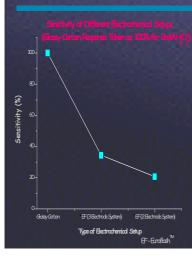
The low sensitivity of the Euroflash<sup>TM</sup> is due to high charge transfer resistance, which is diminished even further when the electrode strip is used independently, i.e. using the inbuilt reference in two electrode mode
