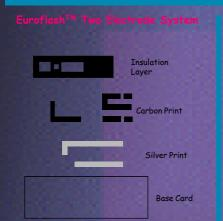
Euroflash<sup>TM</sup> electrodes are fabricated using a screen-printing technique and composed of an Ag/AgCl reference and a carbon working electrode. Electrode areas are defined by an insulating layer.
