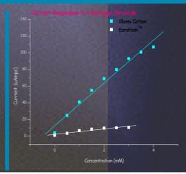
This feasibility study has demonstrated that although the HRP peroxide biosensor works, it is only at its optimum when using a glassy carbon electrode. The next step is to design an electrode strip that meets manufacturing requirements, and that has minimum charge transfer resistance, in order to boost sensitivity.
