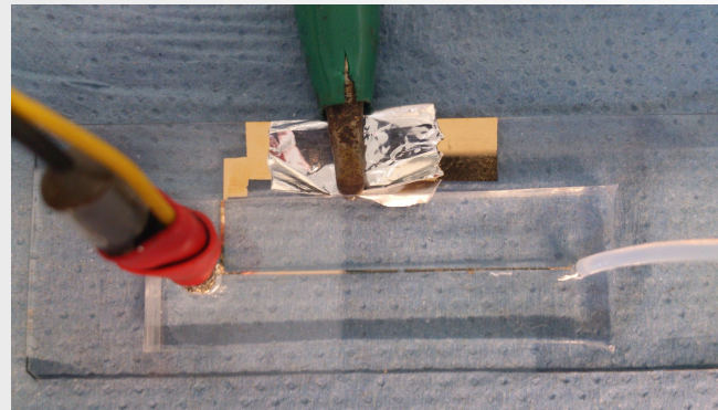
Cross-sectional view of channel outlet housing the reference and auxiliary electrodes
