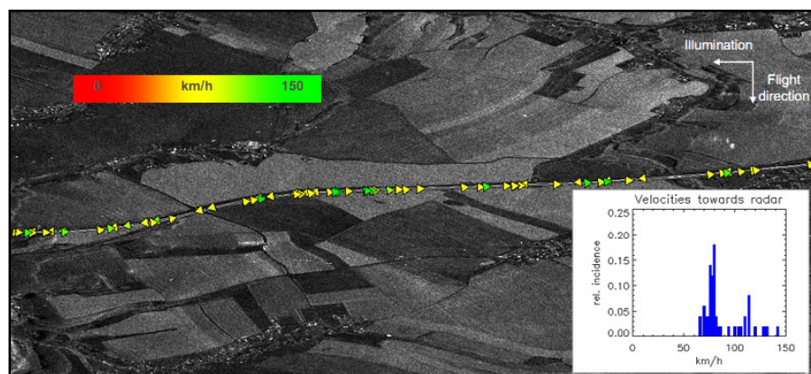
Figure 3.4: TerraSAR-X traffic monitoring on the A4 motorway west of Dresden, Germany [50]
