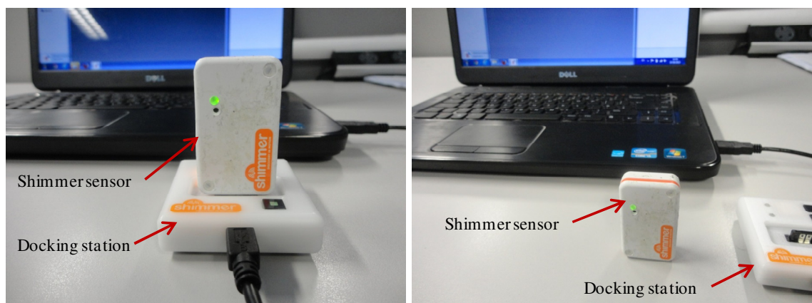
Figure 4.8: Shimmer sensor connected via Bluetooth with or without the docking station
