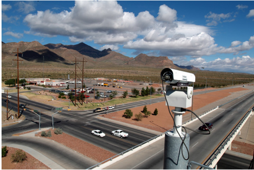
Figure 3.2: Camera-based traffic monitoring system deployed on a roadway [13]
