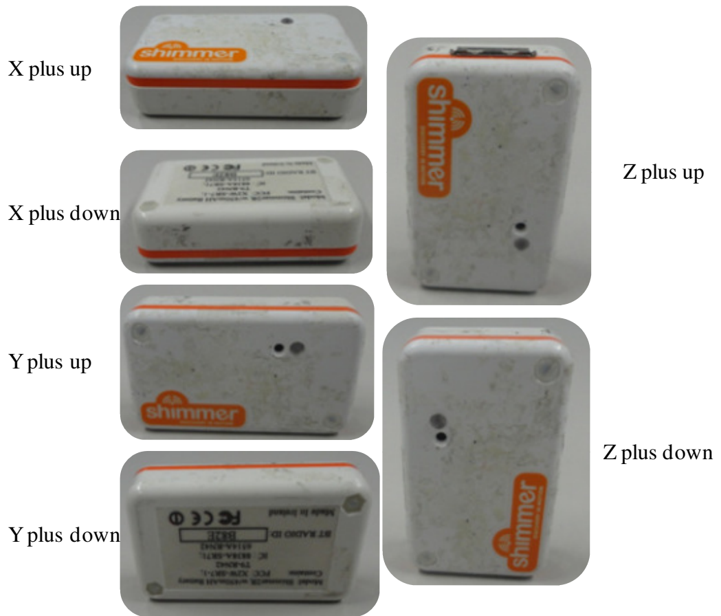
Figure 4.11: Orientations of Shimmer sensor during calibration
