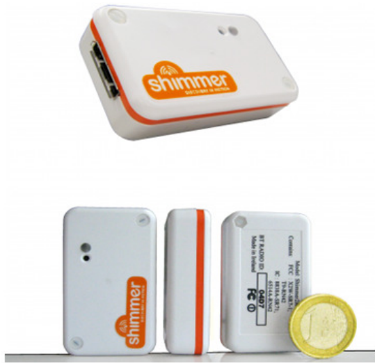
Figure 4.3: Shimmer wireless sensor device [105]
