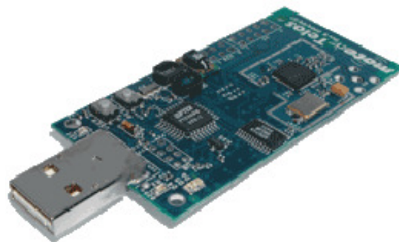
Figure 2.6: A TelosB sensor node [13]
