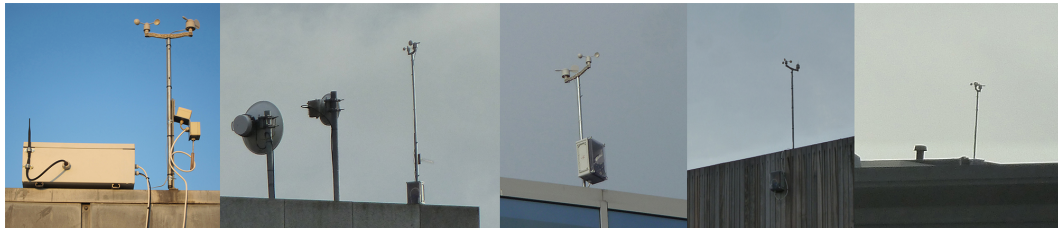
Figure 3.14: Base-station and the five anemometers deployed across the Dublin City University campus
