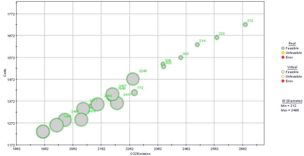
Figure 5.32 Bubble Plot; CO 2 emission and costs of selected results w.r.t. NSGA-II optimiser
