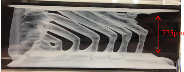
Fig. 5.21: 3D laser blown crystal engraving of dislocation loops from fig. 5.7
