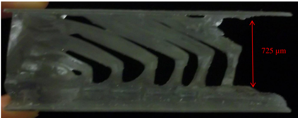
Figure 5.20: Physical representation of the dislocation loops from fig. 5.7. Part created using SLA technology from Advanced Design Consultants.
