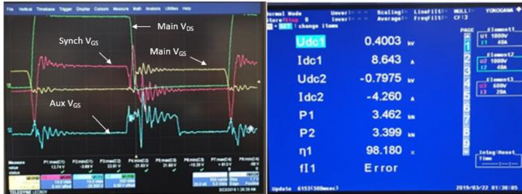
Figure 4.8: Waveforms and efficiency results for 3.3kw module
