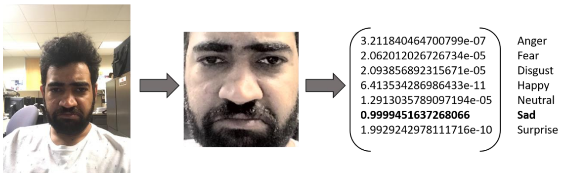
Figure 24: The output produced by the model for images captured using the iPhone camera for sad expression.
