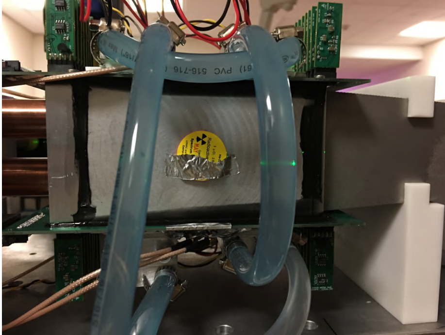
Figure 55: The Na-22 source placed on the detector for calibration purposes. The placement is near the center of each detector so that each channel of the detector can be calibrated for positioning if necessary.
