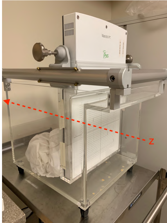
Figure 14: The DigiPhant scanning water phantom which houses the MatriXX 2D segmented ionization detector. The beam axis runs parallel to the shown the z-axis.
