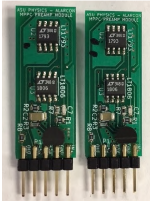
Figure 44: MPPC Preamp Module, designed to plug into headers on the readout board.
