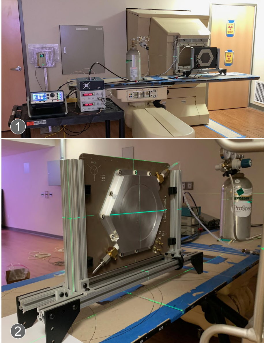
Figure 97: The fluence detector setup at the fixed-beam room at Mayo Clinic in Phoenix, AZ
