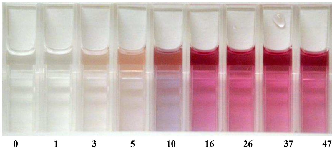
Figure 3.6 Optical images of samples containing different C_{16}TAB and C_{12}TAB concentrations irradiated with a range of X-ray doses (Gy) (A) 2 mM C_{16}TAB , (B) 4mM C_{16}TAB , (C) 10mM C_{16}TAB , (D) 20mM C_{16}TAB and (E) 20mM C_{12}TAB 2 hours post X-ray irradiation. The corresponding X-ray radiation dose leading to the observed visual color change is indicated below each sample in Gray (Gy).
