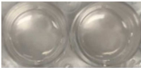
Figure 5.14 Images of nanosensor gels containing irradiated with (i) 0 Gy RBE (control) and (ii) 2 Gy RBE . In each image, C 12 TAB-loaded gels are on the left and C 14 TAB-loaded gels are on the right. Images were obtained after (A) 2 hours (B) 1 day and (C) 1 week post irradiation with protons (or not in case of the control or Gy RBE images). Representative images from n=3 independent experiments.
