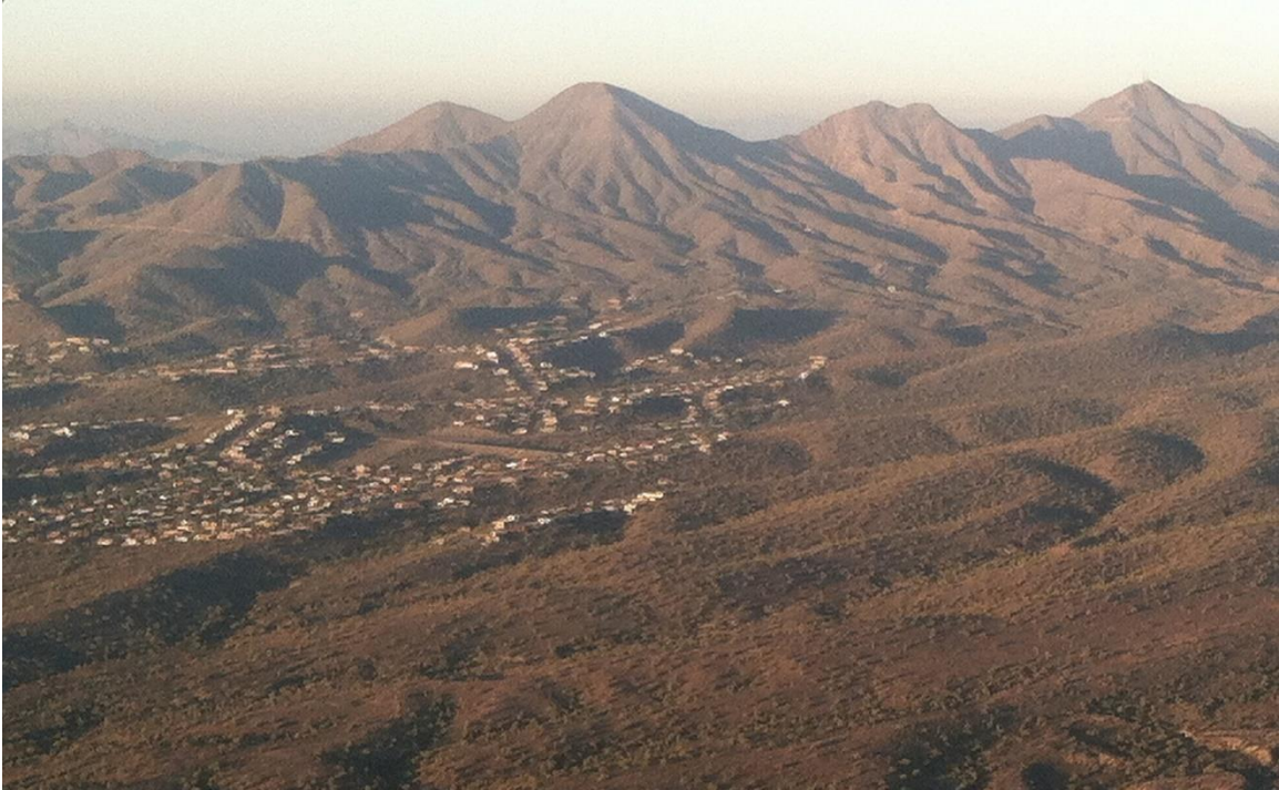
Figure 2.18. Fountain Hills is a community built on a ballena, or eroding alluvial fan. Although structures are safe because homes and businesses are placed on ballena tops and side slopes, roads must be engineered to survive occasional flooding in the washes between the ridges.
