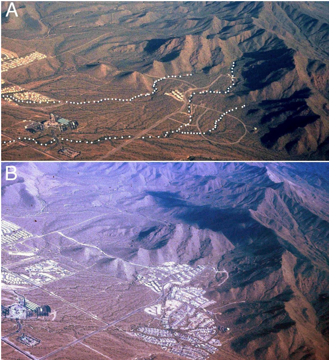
Figure 2.16. Development burgeoned on alluvial-fan surfaces during the 1990s, as shown in a comparison of 1991 (A) and 1995 (B) aerial photographs of the southern McDowell Mountains, Scottsdale. In the 1991 image, dots delineate the presence of entrenched channels transporting water and sediment almost 8 km downstream from this fan. Thus, with the hydrological apex located at distance from the topographic apex of the alluvial fan, all of the development is safe from flooding.
