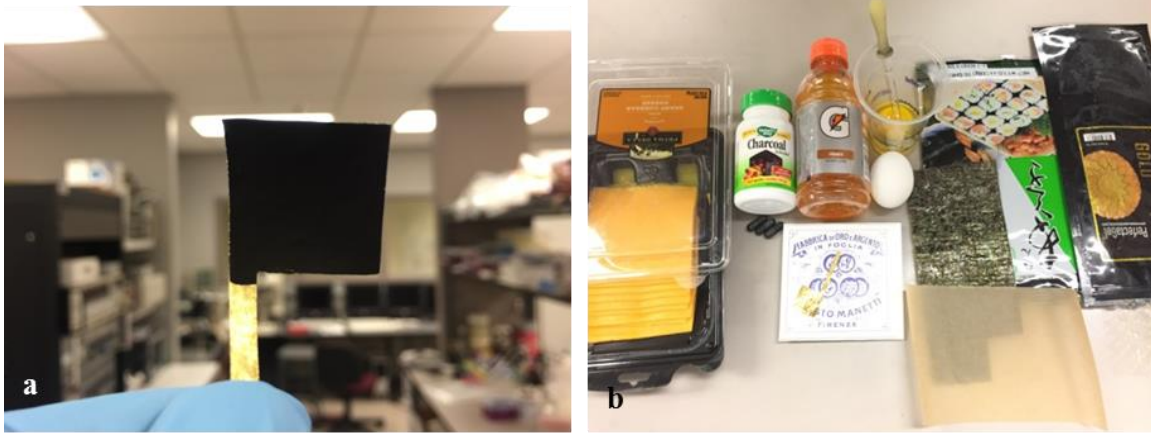
Figure 2.2 (a) Image of a patterned electrode. (b) Material sources for edible supercapacitor, including cheese slices, activated charcoal capsules, Gatorade, egg white, gold leaves, seaweed, and gelatin sheets.
