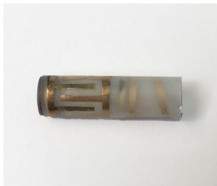
Figure 4.9 Photograph of pH sensor version 2
