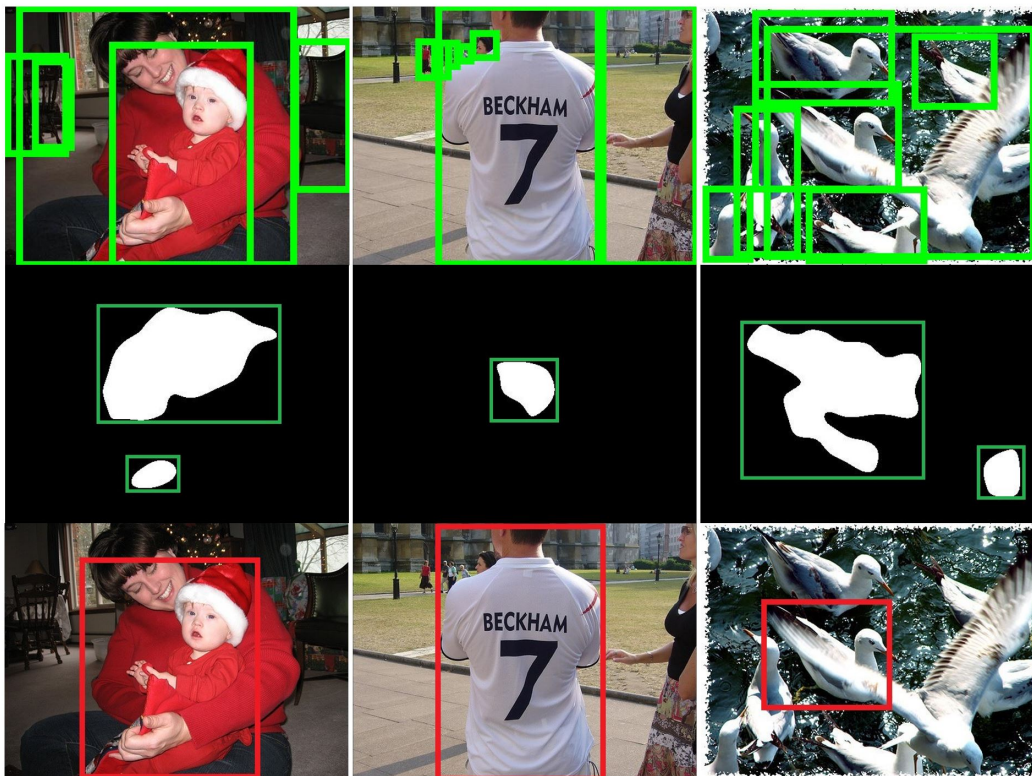
Figure 3.4: Generation of Salient Ground-Truth Objects (SGTOs) From Provided Ground-Truth Objects (GTOs). From Top Row to Bottom Row: Three Sample Images From the PASCAL VOC 2007 Test Dataset with Corresponding GTO Bounding Boxes; Binary Maps Generated by Thresholding the FES [11] Saliency Maps, and Corresponding Salient Regions Bounding Boxes; Images with Salient GTO Bounding Boxes.
