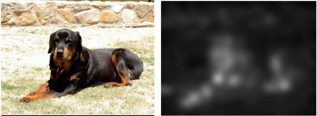
Figure 2.13: BMS Saliency Illustration. (Left) Sample Image from the PASCAL VOC 2007 Test Dataset. (Right) Saliency Map Generated Using the BMS saliency Method.
