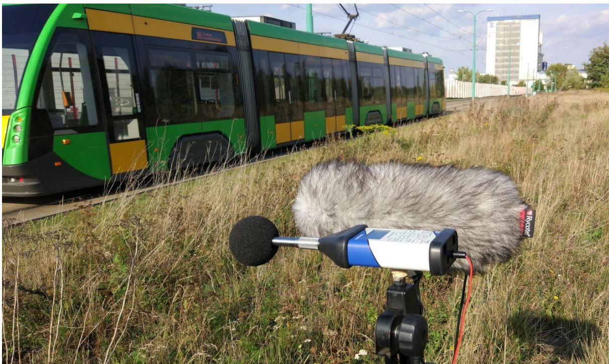
Figure 14. The ambisonic microphone with the sound meter placed nearby during the procedure of recording trams from the distance of 10m.
