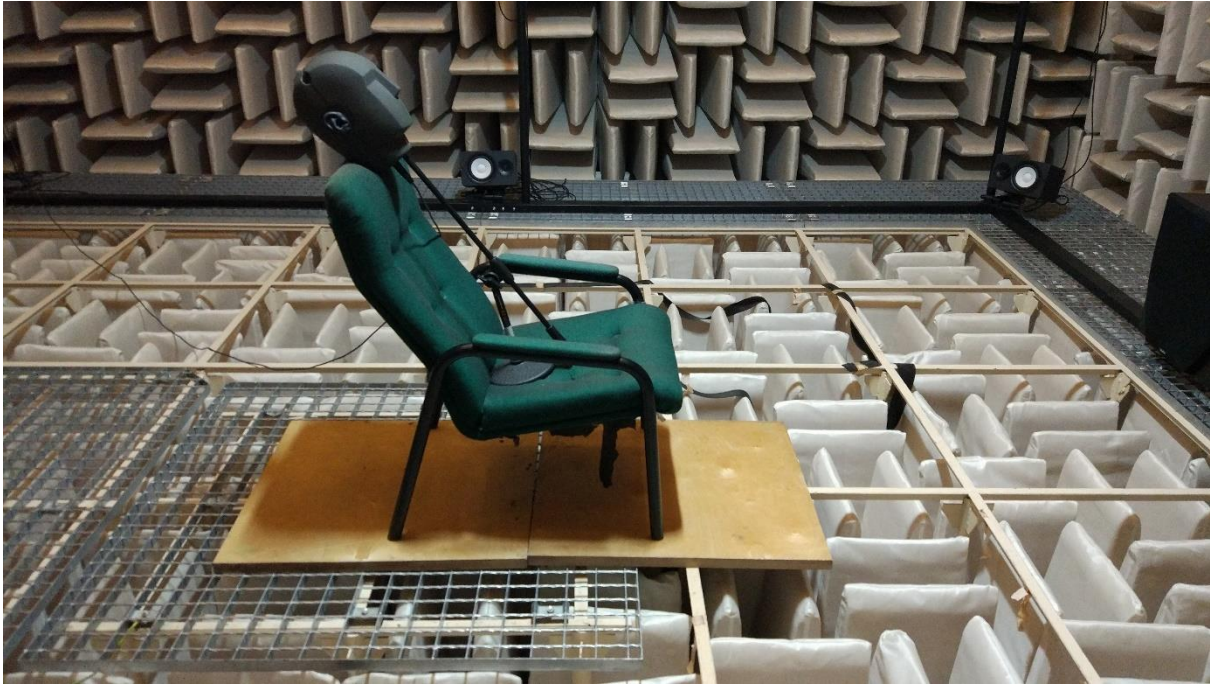
Figure 26. Configuration in an anechoic chamber while recording noise scenarios to stereo signals.
