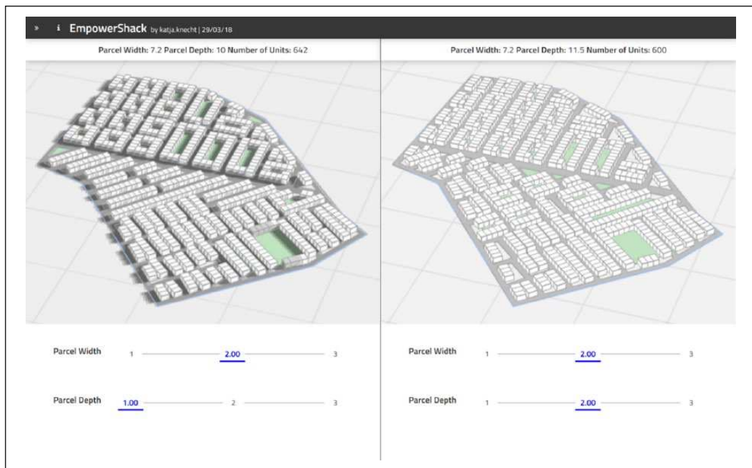
Figure 14. Exploring design alternatives in the beta.speckle online viewer.
