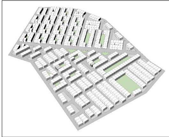
Figure 13. Placement of basic building masses on generated parcels.
