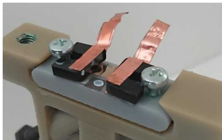
Figure 5.4 Close-up view of the IDT-chip arrangement.
