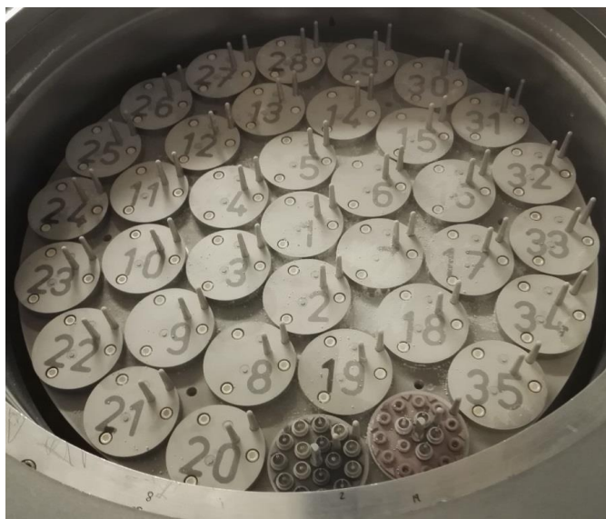
Figure 1.10 Operational beam-side LN2 cryogenic-dewar containing Uni-puck spine holders in positions 36 and 37.
