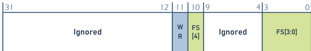
Figure 4.2: Fault Status register masked bits. The FS bits describes the fault status and the WR bit describes the type of the instruction (Write or Read).
