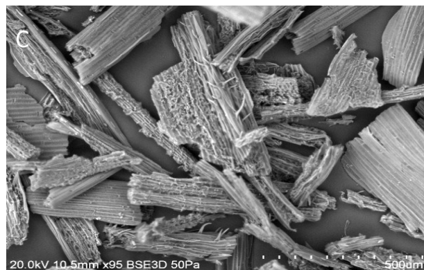
Fig. 1. SEM images of Ground Grass (A) without treatment (B) treated with HCl at pH 4 (C) treated with NaOH at pH 10.
