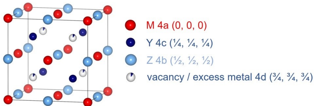
Figure 1.17. Schematic representation of the half-Heusler crystal structure.
