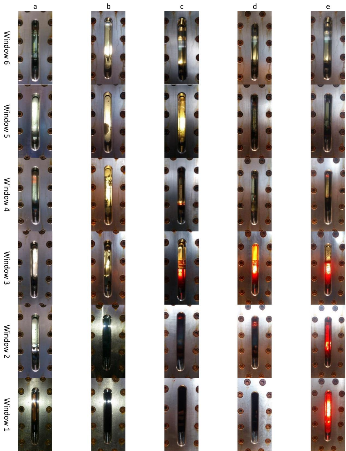
Figure 5-10. Hydrate formation and dissociation, hence hydrate blockage removal during gas methanol injection at 4.5 °C and ~81 bara. (a) no hydrate present, (b) blocked windows with hydrates before methanol, (c) 18 mass% methanol, (d) 26 mass% methanol, (e) after depressurizing to 34 bara.
