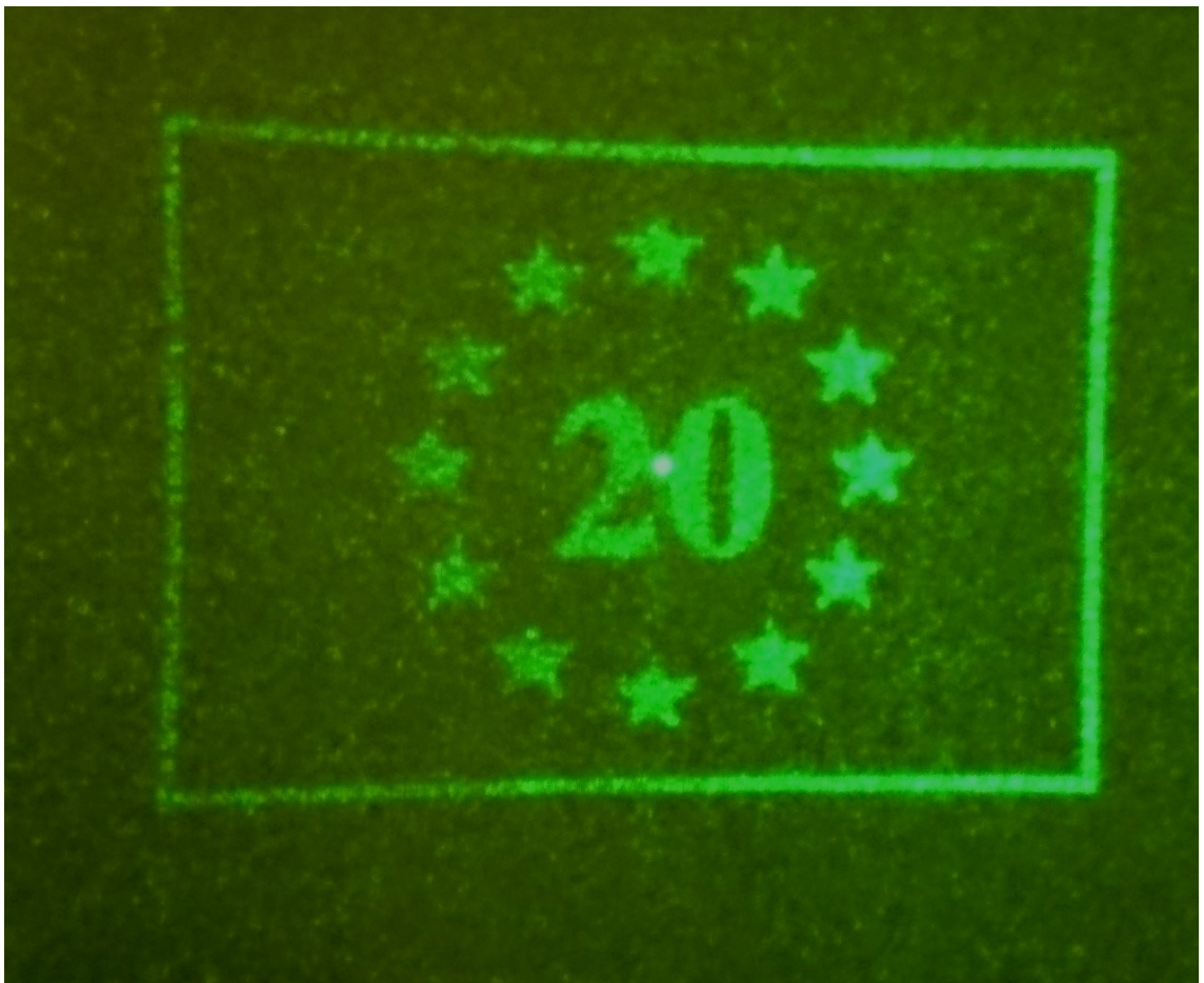
Figure 6.5. Optical output from the -1st diffraction order produced by illuminating the grating at the Bragg incidence angle and projected on a screen. The image appears distorted being captured and projected at an angle.
