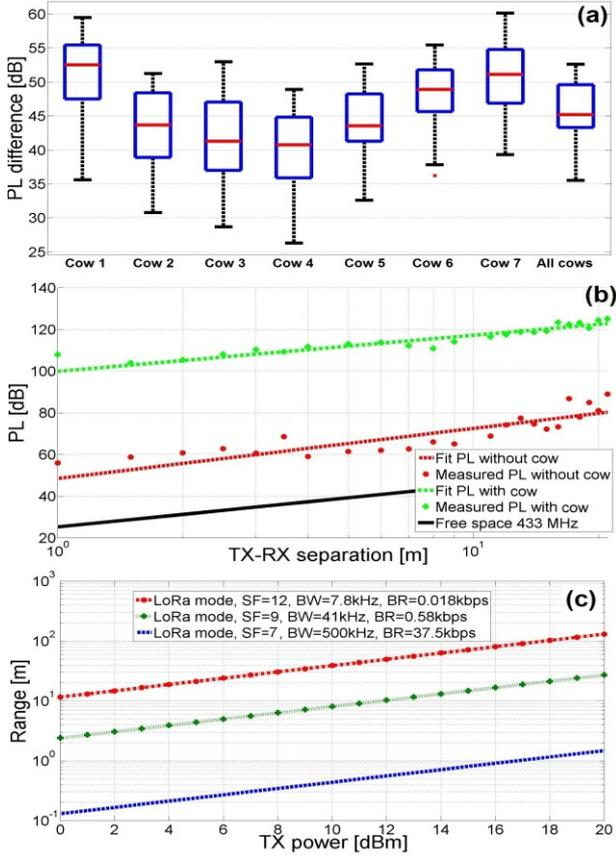
**Fig. 2.** (a) Boxplot of the path loss increase due to the cow body for each individual cow and the average along all cows, (b) the path loss models for the two scenarios (with and without cow) and (c) the calculated network ranges for minimum, typical, and maximum bit rates (0.018, 0.58, 37.5 kbps), SF: spreading factor, BW: bandwidth, BR: bit rate.
