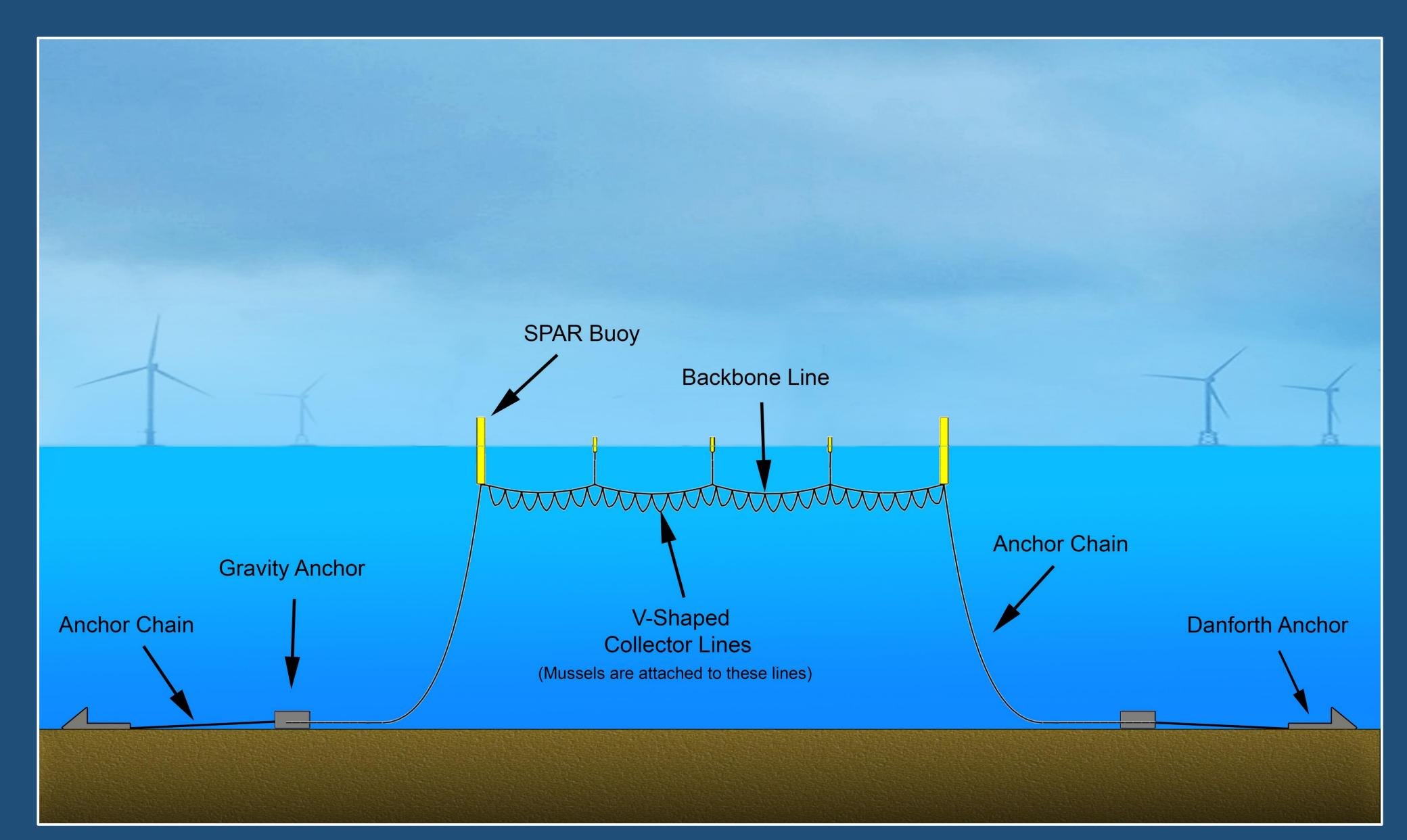
Illustration of a semi submerged longline system that is considered for the study. The floating system consists of a long backbone line, several buoys along the backbone and collector lines to which mussels are attached. At each side, a SPAR buoy is connected to a gravity anchor with a chain. Another chain connects a gravity anchor to a Danforth anchor (length not drawn to scale).
