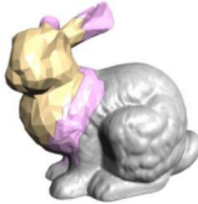
Figure 7.1: Example of simplification using processing sequences. This snapshot shows the yet unprocessed part of the input data (grey), the current in-core portion (pink) and the already decimated output (gold). Courtesy of [ILGS03]
