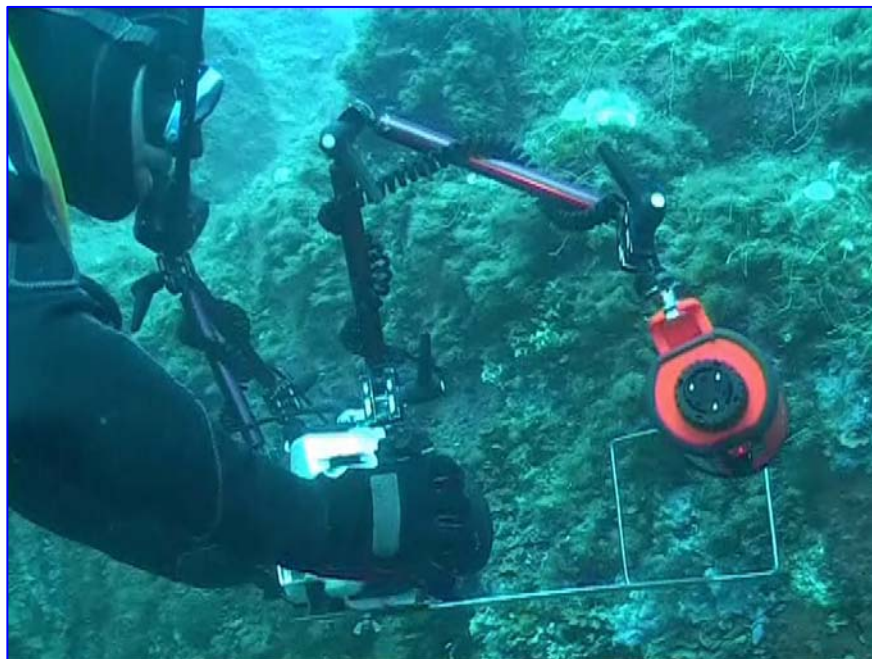
Figure 4.2: Researcher (myself) using the camera equipped with frame and flashes to record the studied substrata.
