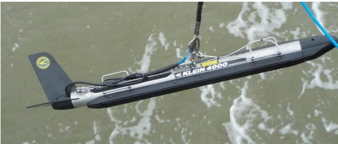
Figure 5.1: Towfish of the Klein System 4000 sidescan sonar. The transducers are mounted at both sides of the towfish.
