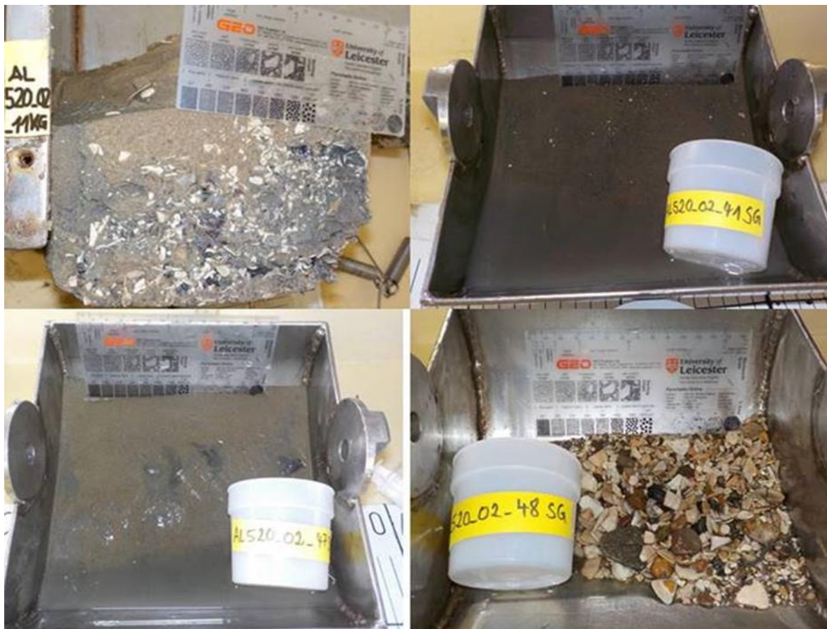
Figure 5.10: Photos of sediment samples. Most sediments consist primarily of fine sand with varying amounts of mud, medium sand, and gravel. One sample (lower right) mainly consists of gravel. The amount of shells varies between <5% and ca. 40%.
