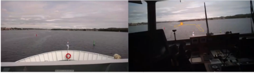
Fig. 8: Eye-tracking of the manual look-outs fixations. Left: Forward facing camera used as reference in the analysis. Right: Eye-tracking result. The yellow spot surrounded by a thin red line indicates fixation on an object.
