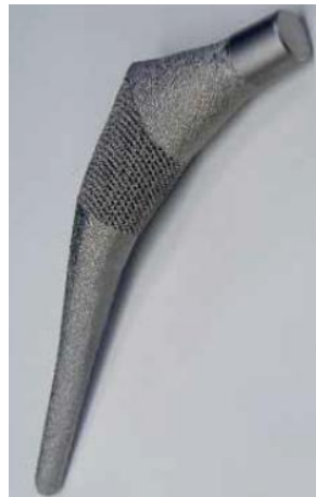
Figure 15 EBM hip prosthesis stem(Ferrís-Oñate, Morales-Martín et al. 2010)
