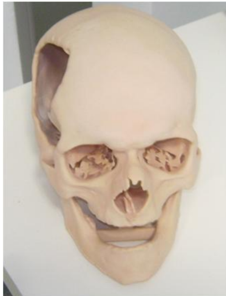
Figure 14 SLS skull patient specific biomodel (courtesy of BRECA Health Care)
