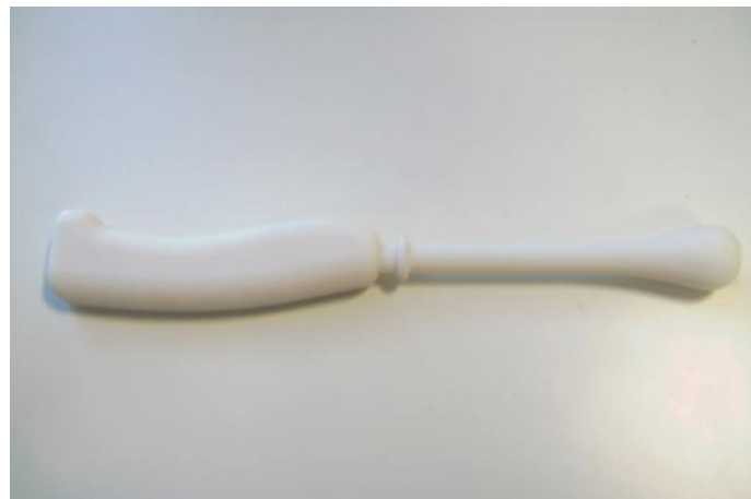
Figure 12 An SLA model of a medical an ultrasound device (courtesy of END Lab University of Granada)
