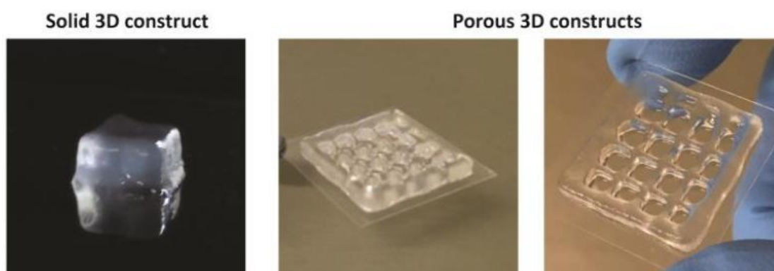
Figure 67 Printing of methacrylate modified pectin bioink
