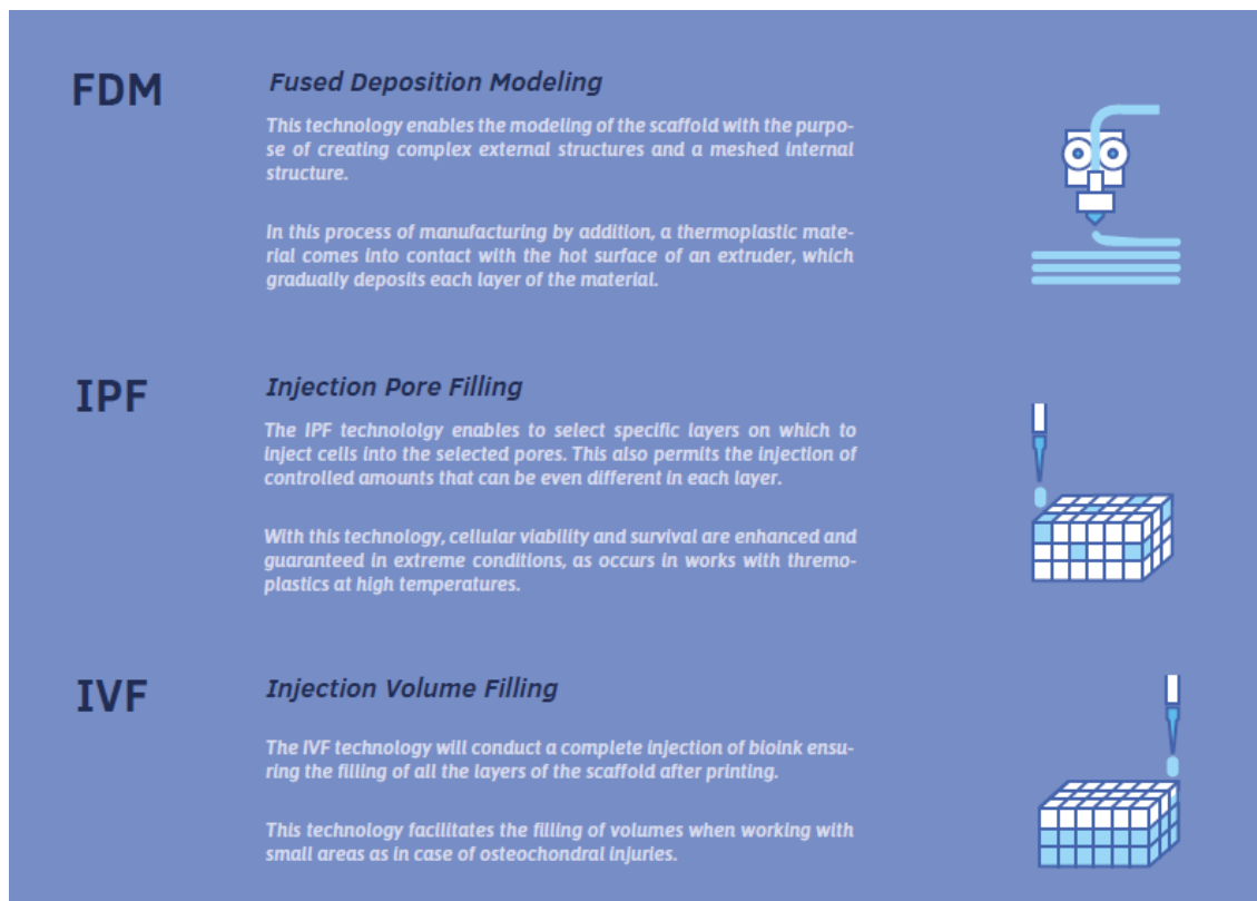
Figure 27.3 Main manufacturing modes that can be used in the system
