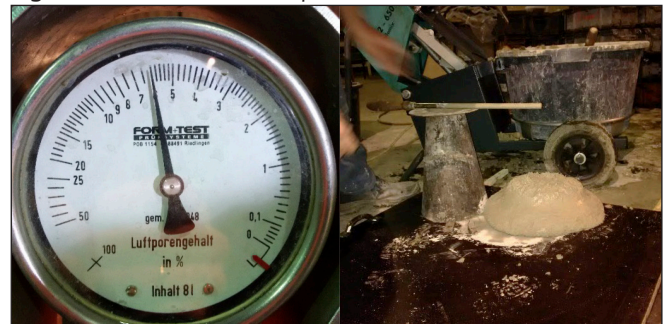
Figure 3. Air content and slump test
