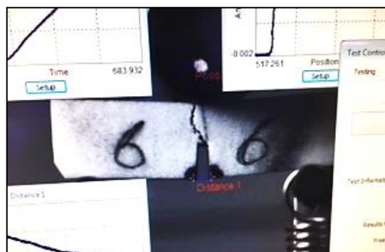
Figure 3-17. A ceramic/polymer interpenetrating phase composite specimen at the end of the fracture toughness testing procedure.
