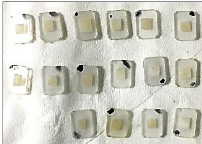
Figure 3-13. The final enamel specimens prepared, polished and set in epoxy resin. Specimens were marked with a spot for orientation during testing.
