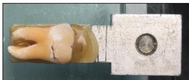
Figure 3-10. Tooth fixed to holder by wax prior to cutting.
