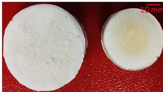
Figure 4-8. Typical porous ceramic specimens before and after sintering respectively. Specimens obtained from initial solid ceramic loading of 30 vol.% through directional freeze-casting and subsequently sintered at a temperature of 1600°C for 2 hrs.
