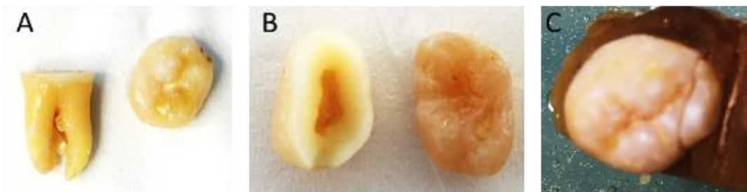
Figure 3-12. Tooth after cutting. A. Crown and root separated. B. The tooth pulp removed. C. The tooth crown fixed to holder by wax after specimen was cut.
