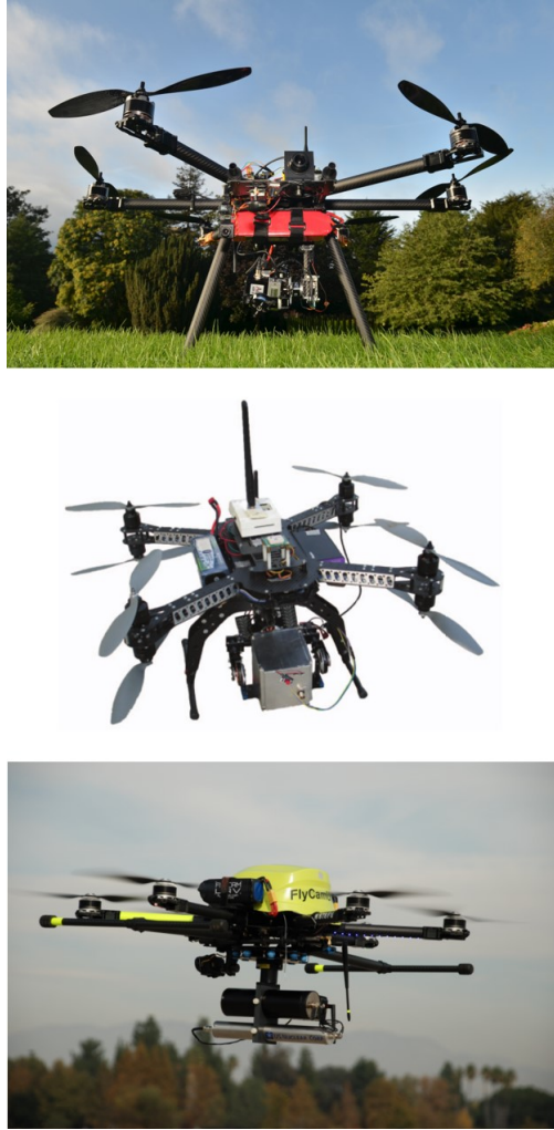
Figure 2.7: Images of typical low-altitude multi-rotor UAV systems employed for high spatial resolution radiation mapping. From (top to bottom) MacFarlane et al., (2014), Aleotti et al., (2015), and FlyCamUAV Ltd (2017) [100, 101, 104].
