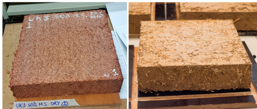
Figure 6. Samples of the manually constructed cob specimen in Plymouth University. The cob sample to the left uses UK subsoil in the mix, while the right one uses French subsoil.
