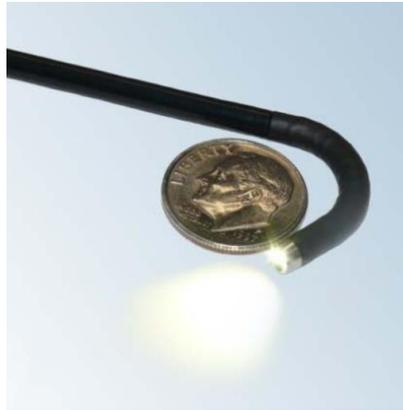
**Figure 4.5:** An endoscope including a commercial leached fibre bundle fabricated by Schott [73].
