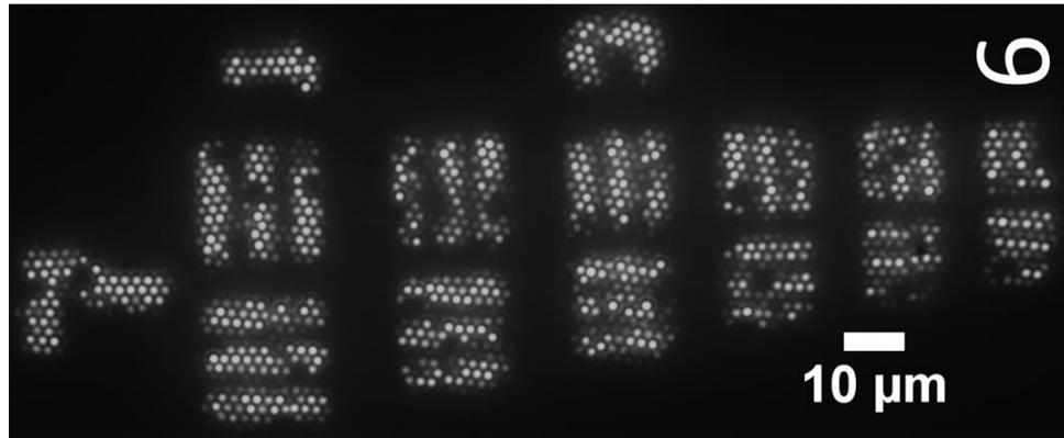
**Figure 6.25:** An image of group 7 of a USAF test target taken using the high resolution 335  $\mu\text{m}$  outer diameter air-clad fiber and a 500 nm bandpass filter. A scale bar and an identifier for element 6 have been added.
