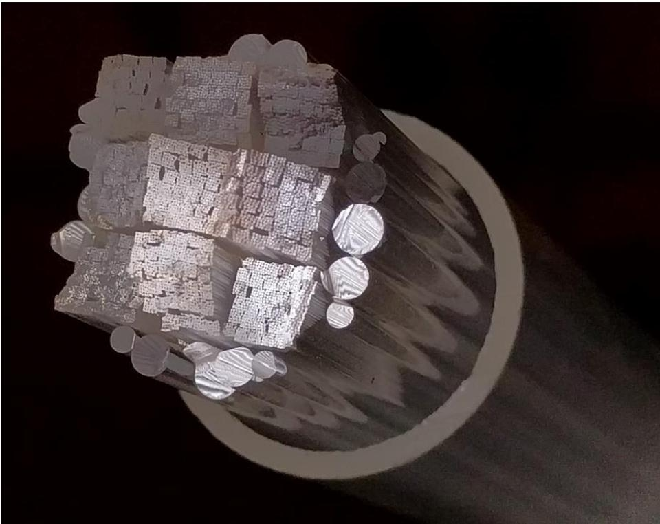
**Figure 4.26:** A square array fibre stack ready to be drawn to preforms or fibre. 9 imaging canes can be seen supported by 4 sets of 5 packers inside a 22 mm OD jacket tube.
