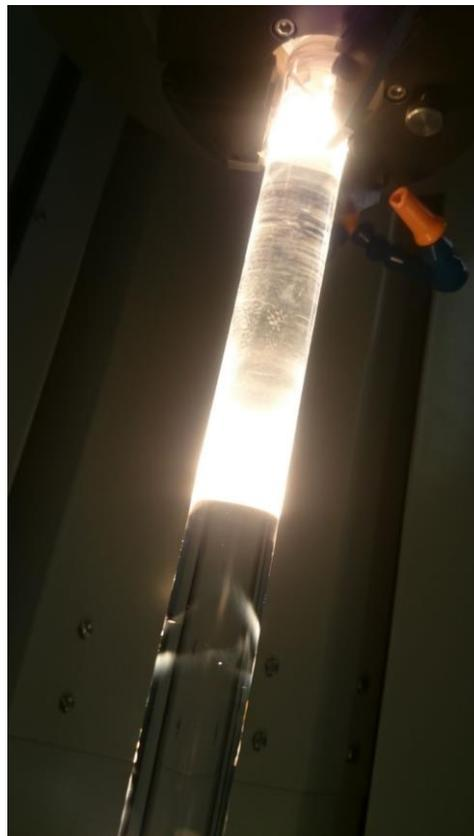
**Figure 4.23:** A graded index preform, lit from below by the furnace. The lower part has been flame polished to remove the surface imperfections that are causing the scattering seen from the top part of the preform, and weakness in the resulting fibre.
