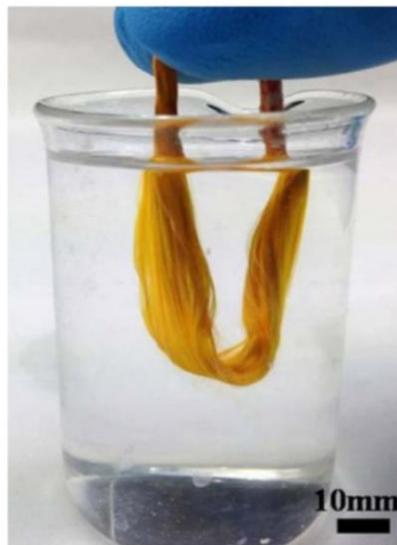
**Figure 4.4:** A soft chalcogenide glass fibre bundle fresh from having its polymer cladding leached away in a solvent bath. It is shown here partially submerged in water [72].
