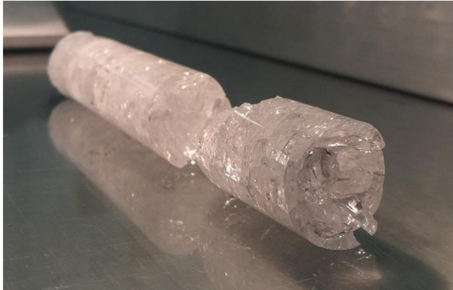
Figure 4.2: A shattered stub from a highly germanium doped graded index preform with an NA of 0.3. A 250 mm length of the preform was being held in a vertical lathe and fused to a pure silica tube using a hydrogen torch. Stress between the differently doped glasses built up over the previous draws in the furnace and uneven heat from the torch caused it to shatter violently, leaving this stub in the chuck.
