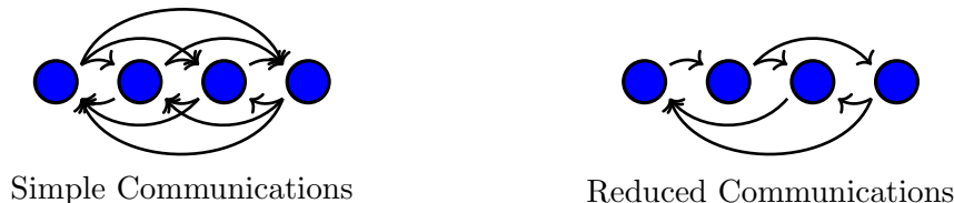
Figure 6.4: An example of reduced MPI communication between four processors (blue circles). Communications are reduced by point-wise cancellation so that communication only occurs in one direction between each pair of processors.
