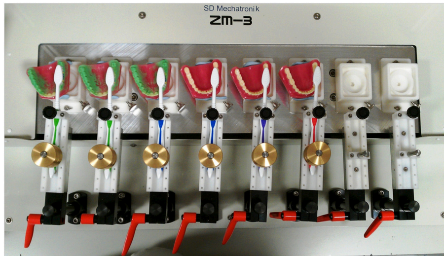
FIGURE 1 | A typical experimental set-up. Up to eight typodonts were coated with simulated plaque and mounted with brushes on the brushing simulator. Typodonts were brushed with a constant brushing pattern under constant pressure for a specified period of time. Typodonts were then photographed and the images analyzed to quantify removal of plaque.
