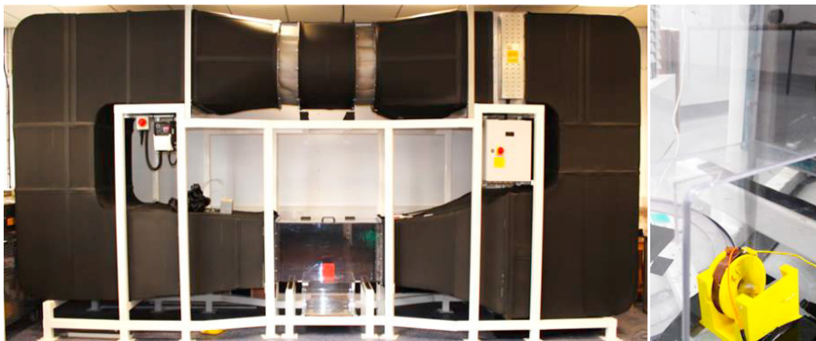
Fig. 2. (a) Side view of the closed-loop wind tunnel (b) WIFEH prototype with one coil configuration showing flutter motion at 2.3 m/s
