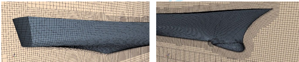
41 Figure 5: Mesh refinements around bow and stern regions.
