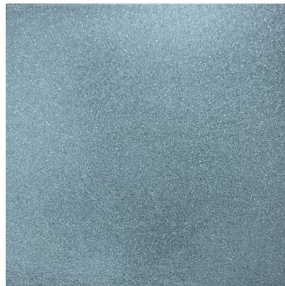
Figure 1- Shot Blasting Profile of samples
