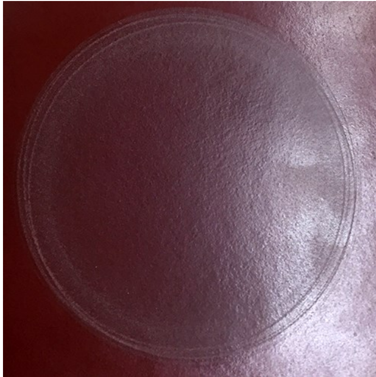
Figure 22 - Epoxy A IN7 sample after 10.000 rounds of abrasion testing on pulsating abrasion tester.
