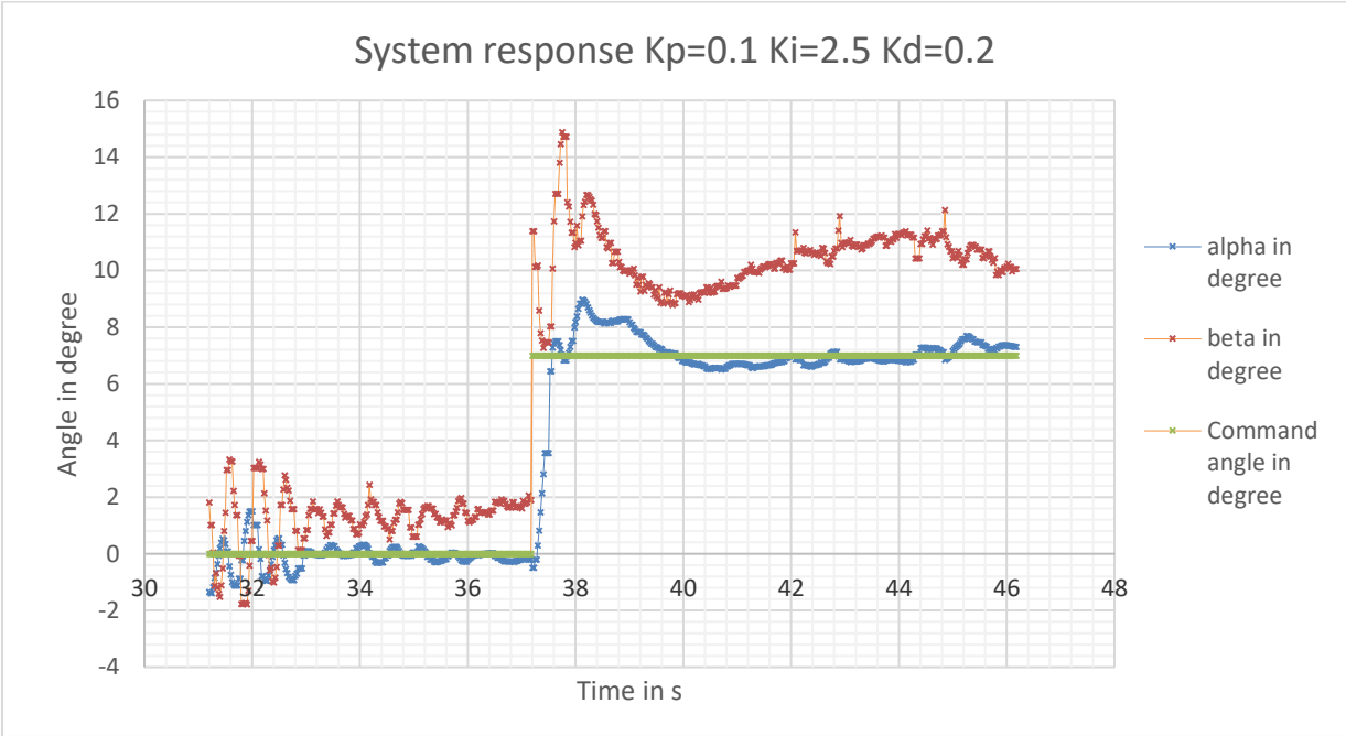
Figure 10-23 System response with a PID controller tuned using Matlab®
