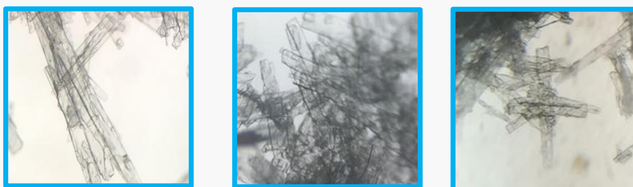
Figure 5. Images under microscope (4X) showing transparent needle-like morphology of the MNYAD_1539 after recrystallization from ethanol. The melting point is 80 °C and this yellow sample has rubber matting-like smelt. These images are first reported for this compound.
